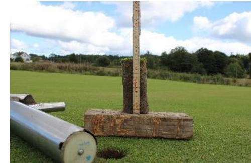
Fig. 2: Measurement of rooting depth at Landvik-NO
